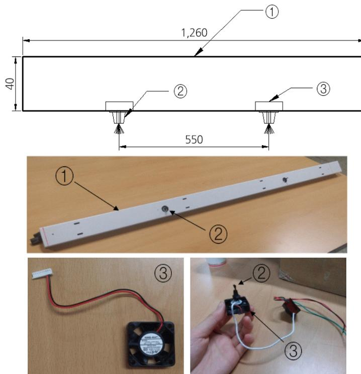
Fig. 1. Anion generation system. ① Case of anion control system ② Anion generator ③ Air blower.
